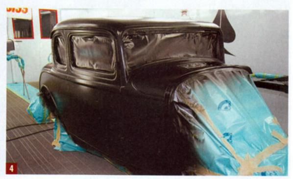
A PPG black base color was shot on the body before the silver Roth 'flake was applied as a base for the candy. The black base made it easier to see when the 'flake completely covered the body.
