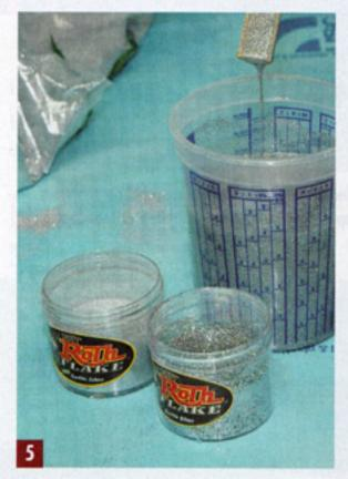
Once the black base was dry, it was starting to get exciting as Shaun started mixing the silver Roth 'flake in the PPG clear. Shaun mixed two parts of the finer 'flake and one part of the bigger 'flake in the clear to get a better covering faster.
