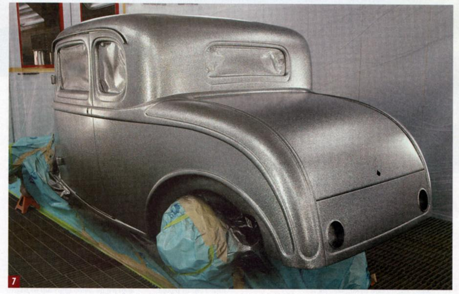
The body started to look impressive with the glittering Roth 'flake after three or four layers, but we could still see some black between the 'flakes upon closer inspection. That called for more layers.
