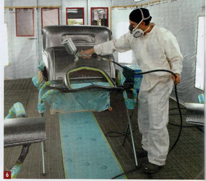
Shaun sprayed the first layer of the Roth 'flake on the body with a big 2.2mm tip in the gun and the clear/'flake mix unreduced. All the parts should be sprayed at the same time to keep the layers and color the same. We masked off some areas (like inside the grille shell) to avoid too thick of a buildup that might prevent pieces like the grille insert from fitting.
