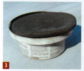
We used a guidecoat powder instead of paint for the final block sanding with 320-grit because most of the sanding was done at this point and we wanted to avoid getting too heavy of a guidecoat. The powder wipes on, leaving a very thin coat that shows minor imperfections and sanding scratches.
