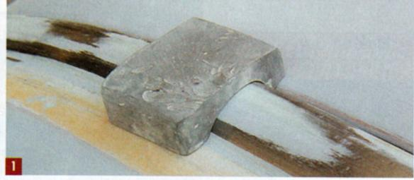
To ensure the rear body reveals that run along the decklid were as straight as we could get them, we made a sanding block from All-Metal that fit the shape perfectly. A little piece of fine-grit sandpaper was then used in it to sand the reveals on the car.
