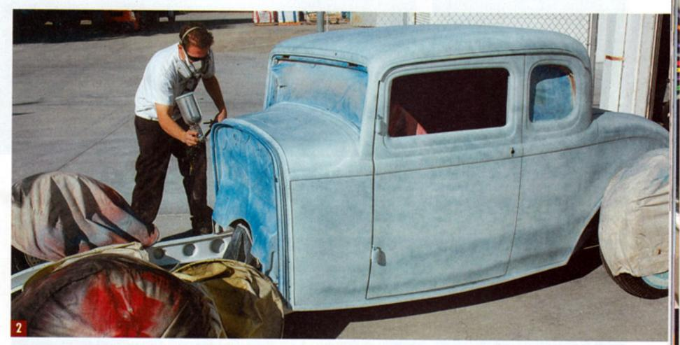
The body was pretty straight at this point, but Ryan Spade sprayed a light guidecoat before the 150-/220-grit sandpaper block sanding began. It was much easier to sand and see what we were doing with the thin coat of color on top of the primer.
